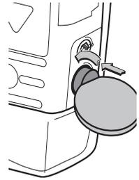
4. Remove the cassette hooks from the pump hinge pins.
