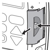
2. Match the + and - markings on the new battery with the markings on the pump. Insert the battery. The pump will beep if the battery is inserted correctly.
