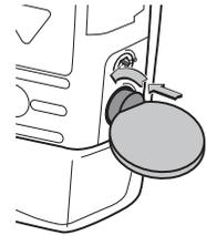
4. If appropriate, insert the pump key into the lock and turn counterclockwise until the white mark lines up with the solid dot. Press **NEXT**.
