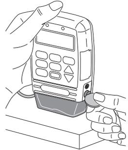
3. Insert a coin or the side of the key into the latch button, push in, and turn counterclockwise until the mark on the latch lines up with the solid dot and you feel the button click into place.
