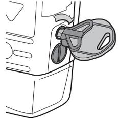
3. Use a coin or the side of the key to unlatch the cassette (the part of the reservoir or administration set that attaches to the pump). Insert the coin or the side of the key into the slot and turn clockwise until the latching button pops out. (The mark on the latch will line up with open dot.)
