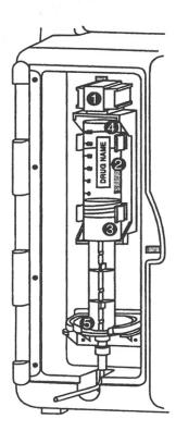
Squeeze Cradle Release Mechanism together at the top of the holder and move to the uppermost position.
