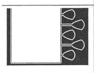
Keys (or Softkeys) are touchkeys which are located to the right of the main display. They perform a variety of functions correlating to the description displayed on the screen.
