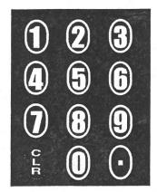
The numeric buttons are used to enter values for any field requiring numeric data.
