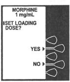
**NOTE:** A supplemental loading dose can be delivered at any time during operation by opening the door and selecting the *Loading Dose*> key. If the 4 (1) Hr Dose Limit is set and has been reached, using the loading dose function may result in exceeding the dose limit.
