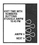
3) Set Time with number buttons. Enter hour as two digits (01:00) and minutes as two digits (01:07 PM). Select AM/PM> to alternate between AM and PM.
