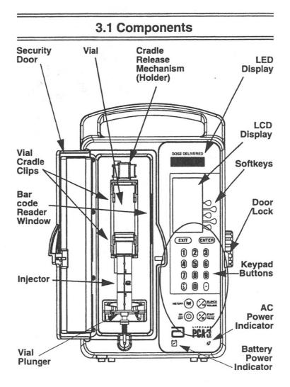
Basic Layout of Front Panel and Keypad
