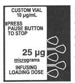
Example screen displaying Loading Dose Value as it infuses. Bottom of screen displays text confirming Loading Dose is active. Upon completion, Red LED (above LCD) displays Dose Delivered.
