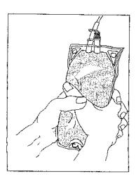
Roll or squeeze the end of the fluid container to force fluid through the tubing and out of the distal (patient) end of the cartridge set.
