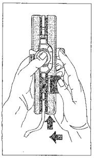
• Push cartridge into cartridge channel until firmly seated.
