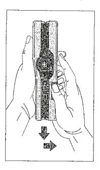
• Open the pump latch by sliding the latch down, then out.
