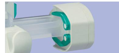
The fixation of the syringe plunger is fully automatic. Herewith unintended boluses are prevented and an excellent start-up characteristic is reached user independently. After the safe fixation of the syringe plunger the piston brake **3** releases. Close the door.
