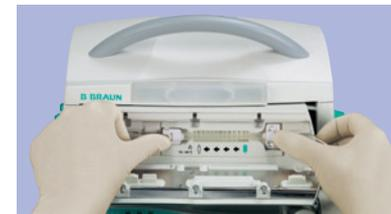
Press **2** to open the door and confirm with "Yes" **3**. Insert the infusion line from right (container) to the left (patient). Insert the two-hole clip of the IV Set in the line guide fixation **1** which is only possible in one direction.
