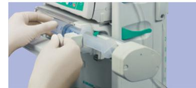
If the display shows the message "Invalid syringe" the wings of the syringe are not properly fixed by the green axial fixation **2**.
