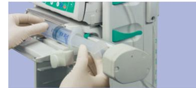
Syringe must be fixed with wings upright in the slot between the green axial fixation **2** and the housing of the pump.
