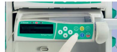
Select the correct syringe brand and type from the list with **⬆** **⬇**. Confirm the syringe type with **OK**.
