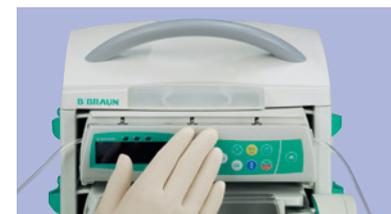
Guide the line through the line outlets of the housing at both ends of the line **9**. Close the door by pressing in the middle of the operating unit.
