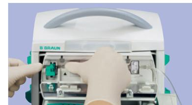
Push the line into the up-stream pressure sensor **6**, the down-stream pressure sensor **7** and the air sensor **8**. Make sure the line has good contact to the surface of the sensor.
