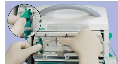
Route the line straight to the finger pump element **2** and click in the clips **3**. Make sure, that you do not twist the line.
