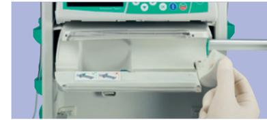
Press **⏻** to switch on the pump. Open the door. Pull and turn the syringe-holder **1** to the right to open the green axial fixation **2**.
