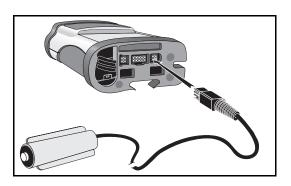
CAUTION: When removing the cord from the bottom of the pump, firmly grasp the connector and pull straight out. DO NOT twist or bend the cord or connector.
