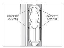
**CAUTION:** Ensure the cassette is properly installed. When properly installed, all four cassette latches are visibly holding the cassette securely in the cassette pocket.
