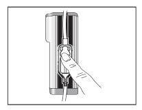
CAUTION: Ensure all four cassette latches are clearly visible after the cassette is installed. Refer to *Loading the Cassette* on page 32.
