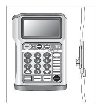
3 Insert the cassette into the cassette pocket by pushing firmly along the entire cassette until it is firmly seated.
