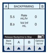
3) Upon release of ▲ [BACK PRIME], the cassette test is performed to confirm readiness for pumping. Pressing (START) will resume programmed delivery.
